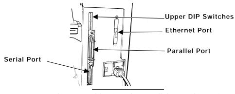
Do not plug any cables into the parallel port when using the Ethernet port.
