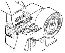
5. Adjust the supply holder guides so the sides barely touch the roll. Make sure the supply roll turns freely. If you are using fan-fold supplies, place the supply stack behind the printer, label side facing up.
