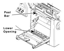
4. Feed the backing paper through the lower opening of the exit cover. Close the exit cover. Pull down firmly on the backing paper to remove any slack.
