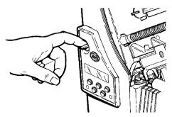
11. Close the printhead by pressing down on the thumb well until you hear it click into place.
