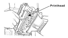
Rub the cotton swab across the supply sensor and die cut sensor and remove any build-up.
