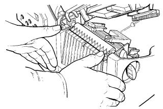
3. Feed the backing paper over the peel bar.
