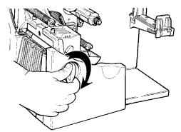
3. Lift printhead assembly using the printhead tab until the assembly locks into place.
