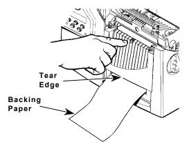
When removing the backing paper, pull up across the saw-toothed tear edge. Make sure the backing paper tears at the edge.
